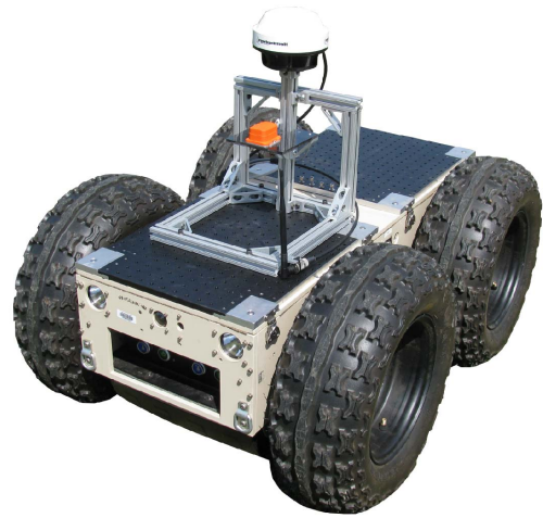
Figure 1: Image of RMP400 robot equipped with sensors required for terrain data collection.
